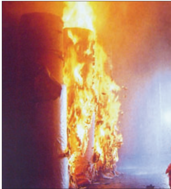
Vertical gaps between the reels and the holes in the centre of reels form chimneys that promote rapid vertical spread of fire
