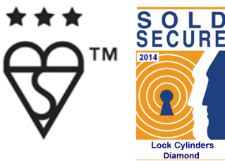
Figure 1: An example of British Standards Institution 3 Star TS 007 cylinder 'Kitemarking' and Sold Secure SS 312 Diamond labelling.
